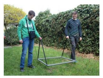
The search frame should be held at a distance between 20 cm and 50 cm (see images) to the ground. If space is over 50 cm it can happen that small to middle-sized metal pieces are not indicated.
