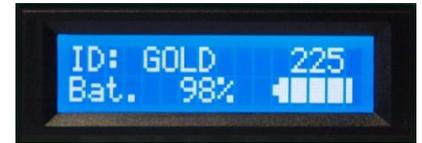
**Note:** The GOLD ID-XL shows a very sensitive reaction towards small gold objects (e.g. nuggets). Through the increase of frequency the depth performance also rises. However, in case of difficult soil conditions an increase in disturbances can occur, which can be reduced by a renewed reset and a reduction in the frequency.
