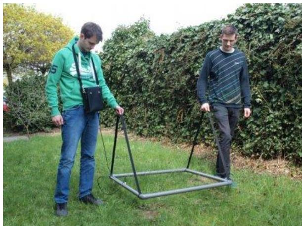
The search frame should be held at a distance between 20 cm and 50 cm (see images) to the ground. If space is over 50 cm it can happen that small to middle-sized metal pieces are not indicated.
