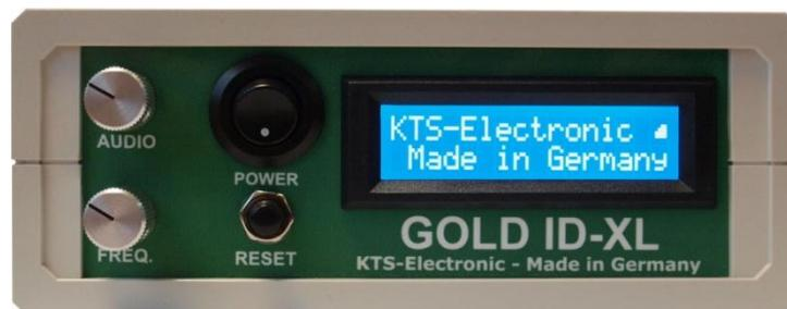
1. Activate the metal detector with the ON-/OFF-button. The respective searchcoil should be cable-connected to the electronic unit beforehand.
