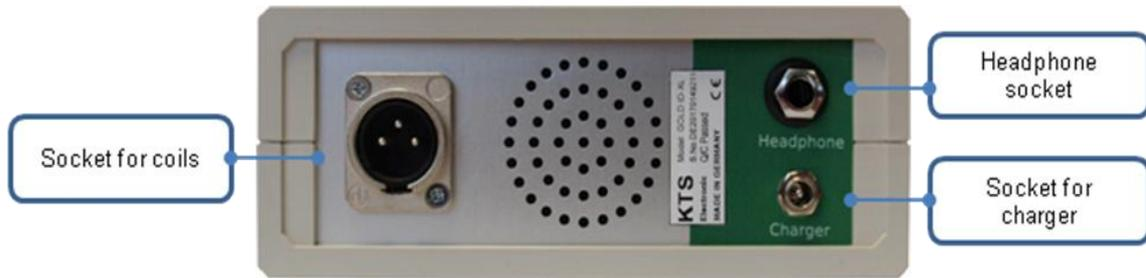
1. **Socket for coils:** The connecting socket for coils is located on the left side. The connector plug of the searchcoil has to be plugged into the socket. Before removing the plug the locking knob must be pressed, only then an extraction is possible. The connector is compatible with all GOLD ID-XL searchcoils.
